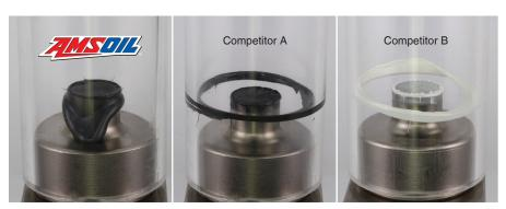
Based on extreme lab testing using a pneumatic test apparatus that applies a controlled, impact-type force on the grease using a ram and anvil. All products tested are NLGI #2. Competitor products purchased January 2020.
