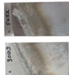
ALUMINUM: Two corroded aluminum coupons showing the effect of CSF. The two coupons were submerged in salt solution for two weeks to build corrosion and salt scale. A sample of CSF was heated to 82°C. The coupons were half submerged for 1 hour (right sides).
