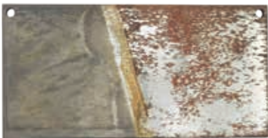
1 HOUR STEEL: A corroded steel coupon showing the effect of CSF. The CSF was heated to and kept at 82°C. The coupon was half submerged for one hour (left side).
