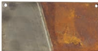
2 HOUR STEEL: A corroded steel coupon showing the effect of CSF. The CSF was heated to and kept at 38°C. The coupon was half submerged for two hours (left side).
